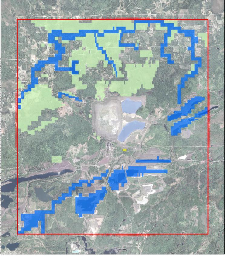
Model Extent Model Grid Model Boundaries Constant Head Cell - Layer 2 Drain Cell - Layer 2 River Cell - Layer 2 River Cell - Layer 1
