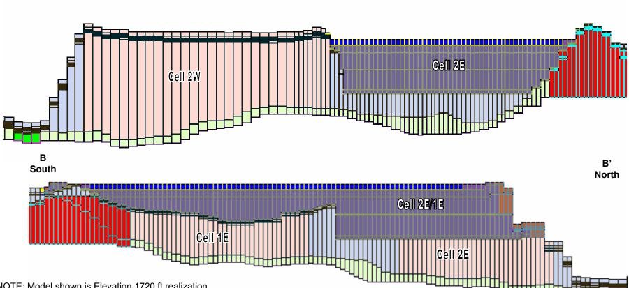
NOTE: Model shown is Elevation 1720 ft realization Horizontal lines define layer boundaries Vertical lines show grid spacing
