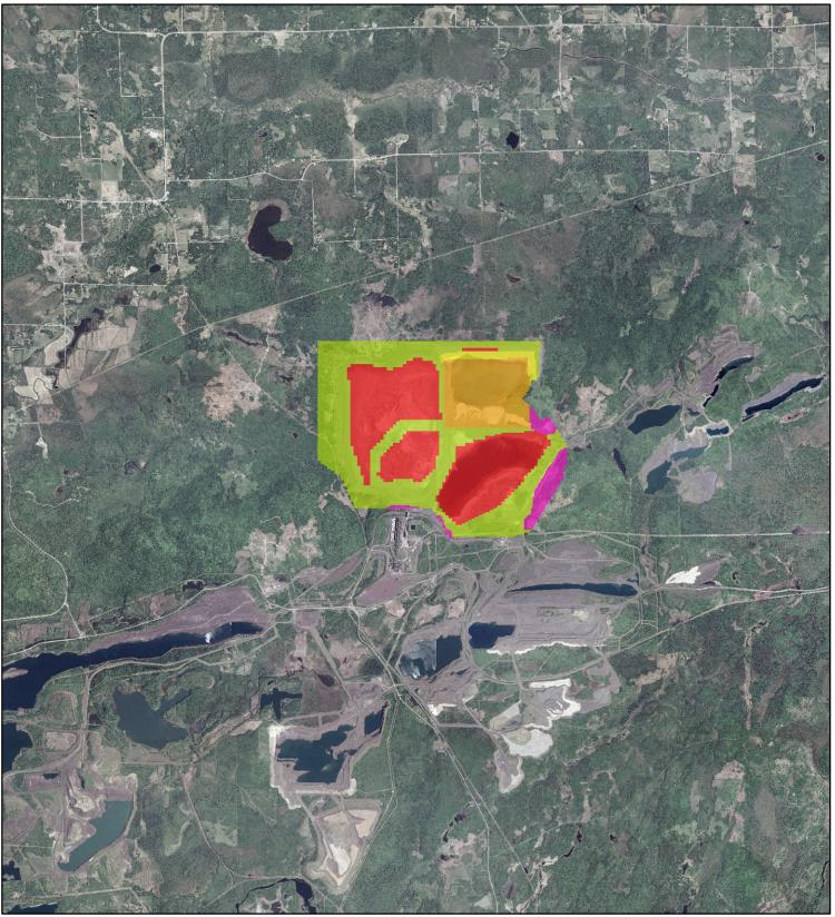
Hydraulic Conductivity (cm/sec) Model Layer 4 8.0 x 10^-9 1.1 x 10^-5 5.4 x 10^-5 6.5 x 10^-5 8.1 x 10^-5
