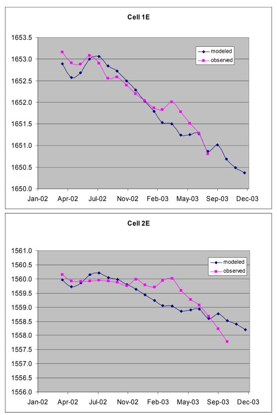
Figure 4-1 Modeled and observed water levels in Cells 1E and 2E for the period of calibration
