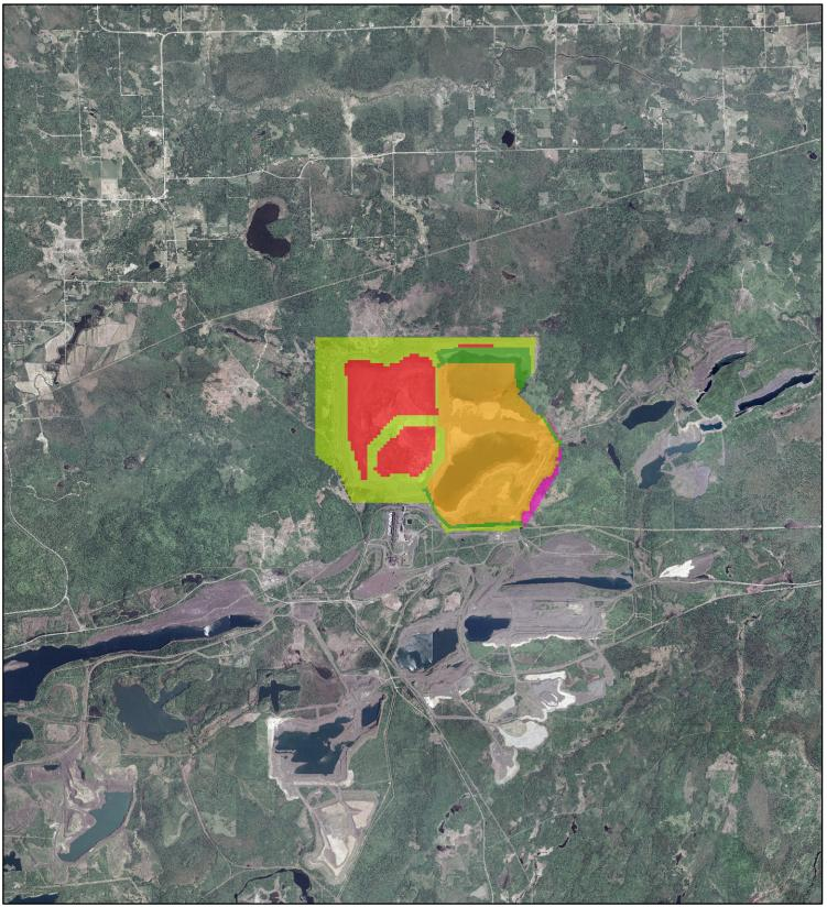
Hydraulic Conductivity (cm/sec) Model Layer 3 8 x 10^-9 1.1 x 10^-5 5.4 x 10^-5 6.5 x 10^-5 8.1 x 10^5
