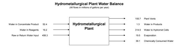
Figure 2 – Hydrometallurgical Plant Water Balance
