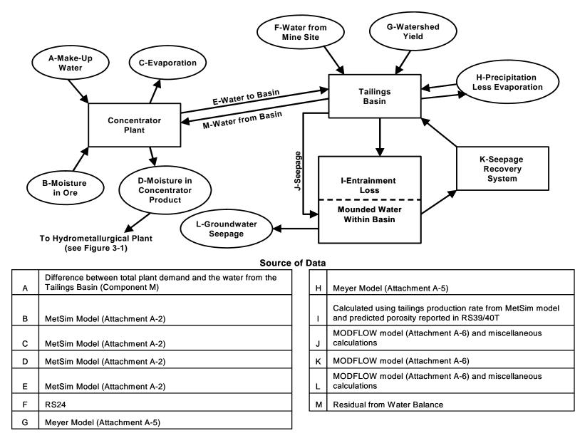
Figure 2-1 Tailings Basin water balance schematic
