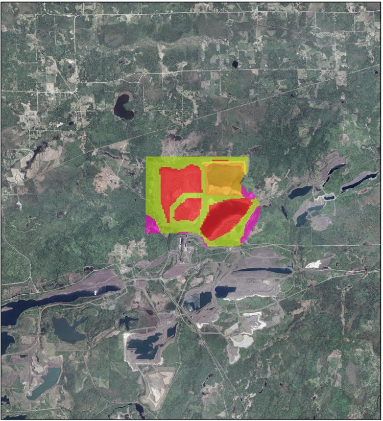
Hydraulic Conductivity (cm/sec) Model Layer 5 8.0 x 10^-9 1.1 x 10^-5 5.4 x 10^-5 6.5 x 10^-5 8.1 x 10^-5
