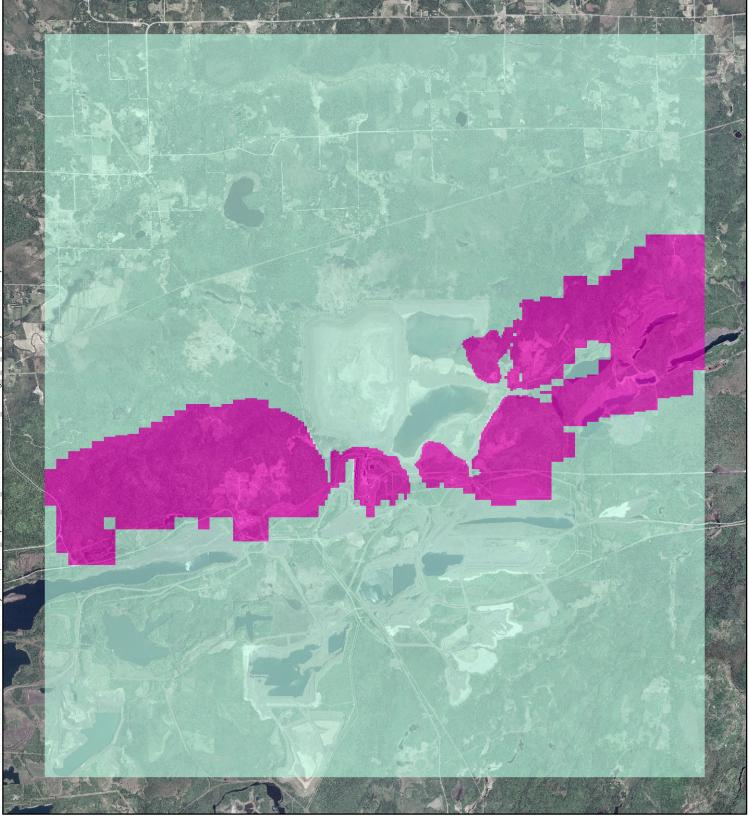
Hydraulic Conductivity (cm/sec) Model Layer 8 8.0 x 10<sup>-9</sup> 2.3 x 10<sup>-2</sup>
